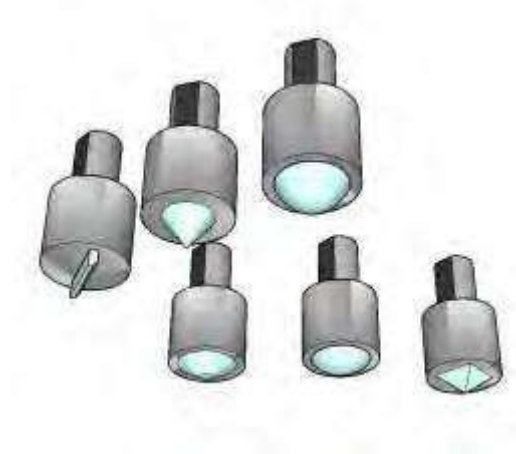
Fig. 3. Appearance and model of indenter's various types
