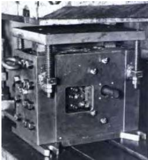
Fig. 1 –Photo of the stamp with the differentiated clamp of the rolled stock
